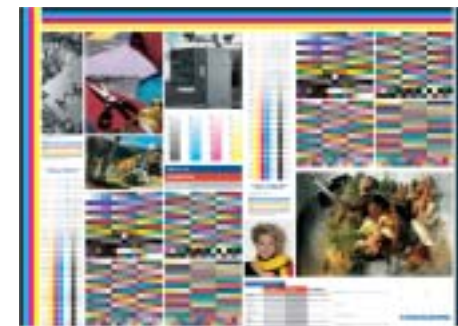
Fig. 21: Typical test print for comparing the actual values of the print with the desired target values of a test file.
